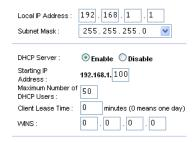
You can let the router automatically assign a dynamic IP address to the computers or devices connected to the network by enabling the DHCP server of the router. In this case, you can access the digital receiver with the IP address which is assigned to the digital receiver by the router.
